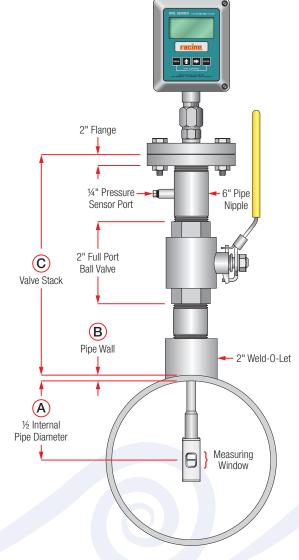
Insertion hardware kits available with flanged or NPT connections.
