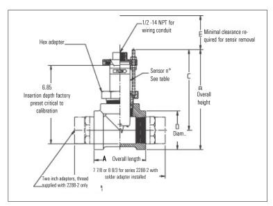
Note: Dimensions "B" and "C" may vary  $\pm 1/4$  inch, depending upon make-up on pipe threads.
